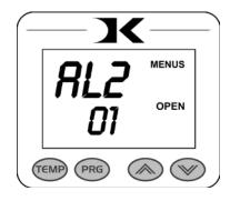
The PPR menu must be set to ON for this menu to be visible. Use the arrow keys to set AL2 to OFF, or 1 through 10.
