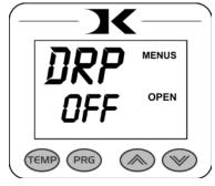
If the current temperature drops below the set temperature by that many degrees, and alarm will sound. Press TEMP to silence the alarm.
